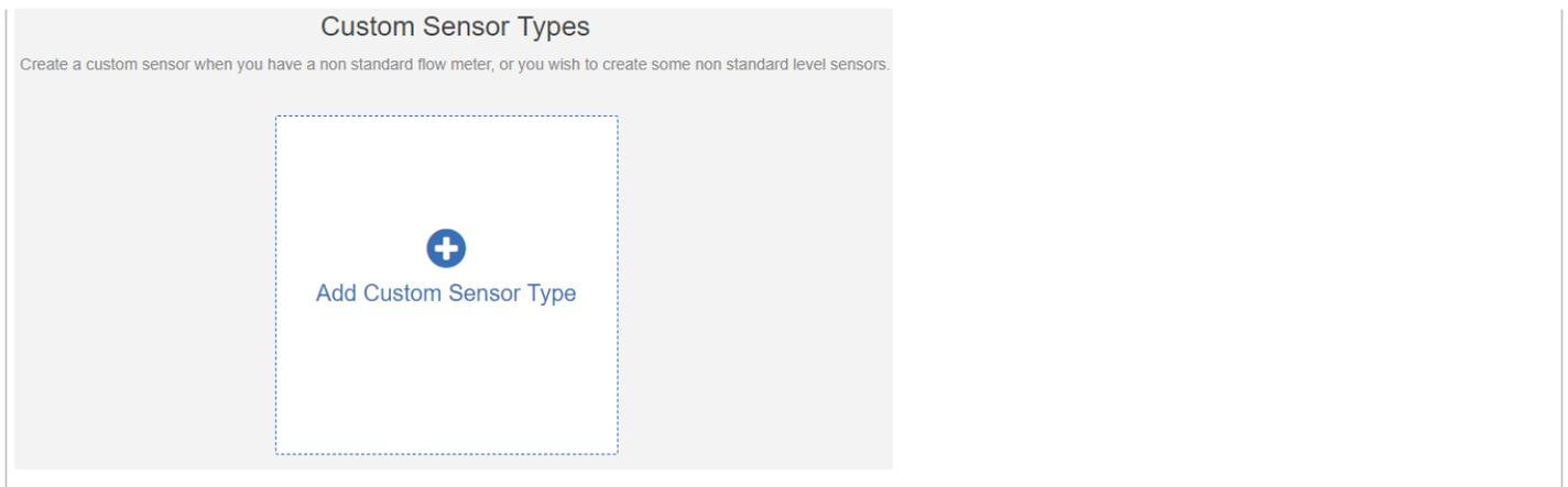
A dialogue box will appear for you to enter your custom flow meter details. Make sure you enter the calibration details for your custom pulse-based flow meter. Please refer to the manufacturer specifications to find out the calibration. Otherwise, you will not get accurate readings to display on your flow data.
